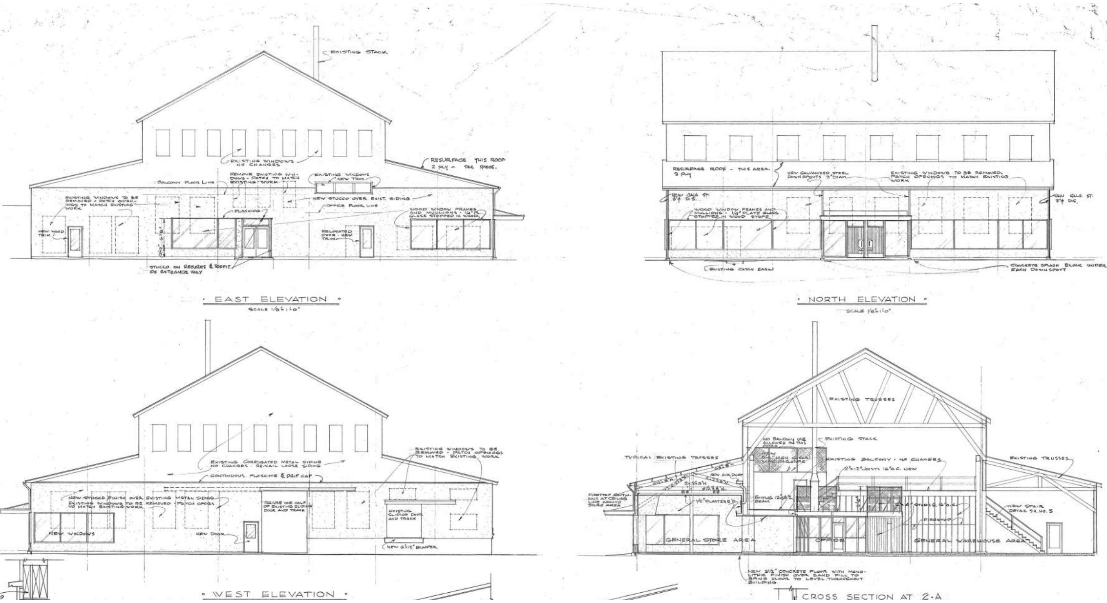
Elevation and section drawings from the 1953 remodel show the changes to the exterior window locations and the addition of interior partition walls to the central high bay space.
